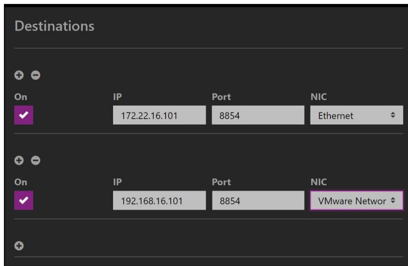
In most situations, the network layer of the operating system can determine based on the target IP address which NIC (network interface, basically which network connector) to use. If you want to explicitly send the data over multiple networks it's not unlikely that an IP address is reachable via multiple connections. To force the encoder to use two different NIC's, you can explicitly specify which NIC to use.
