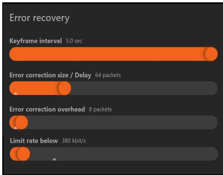
What these settings say is: “Every 64 packets, send 8 extra packets as overhead.”. For each original 64 packets, 72 actual packets are sent. As long as at least 64 of the resulting 72 packets arrive, the decoder can reconstruct all the missing packets.
