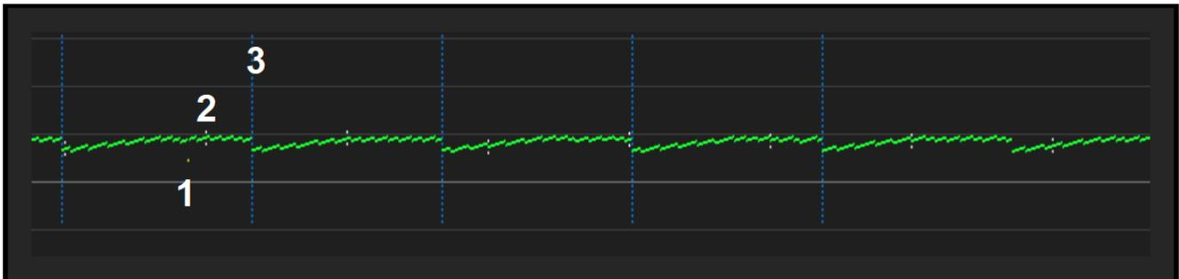
The green pixels indicate that a packet was received without issues. The distance between each green pixel and the brightest horizontal line indicates how much time was left when the packet was decoded, before a drop would have been caused. The thinner horizontal lines indicate seconds, so all the green packets here arrive between about 0.6 and 1.0 seconds before it's too late – which corresponds with a Delay setting of about 1 second.
