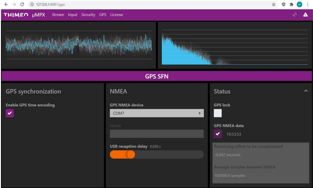
First, the GPS NMEA data will appear. After about 30 seconds, GPS lock will light up (both the name under Status and the GPS symbol in the top right corner of the screen):
