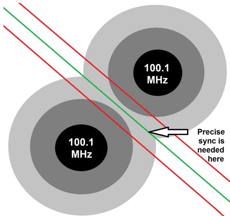
To do this, the MicroMPX encoder needs to add timestamps to the audio, and the decoders all need to precisely synchronize when they play the audio using a GPS clock.
