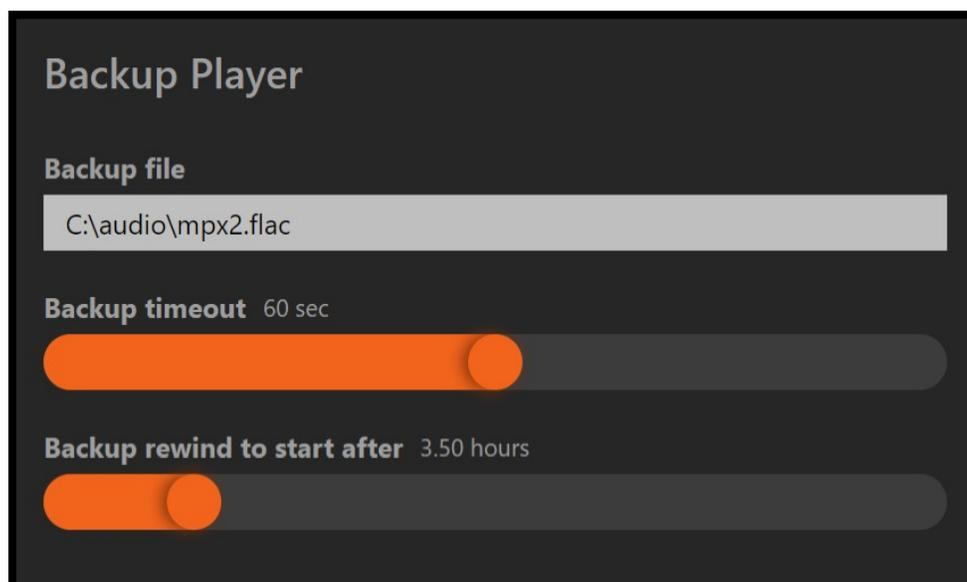
The backup player kicks in after Backup timeout time of no usable MicroMPX data coming in. If a few packets arrive and then the signal disappears again, it will continue the backup file playback where it left off, unless the backup player hasn't been used in Backup rewind to start after time. In that case it will start at the beginning. If you always want it to start at the beginning (for example if you have a loop of jingles as backup file), you can set that time to 0.
